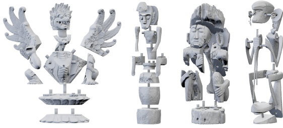
Figure 3 Artifact exploded view of the four assembly models showing segmented parts and joints placement.
